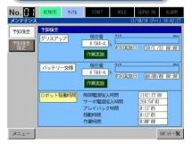
Displays grease-up, battery exchange time management, power on time
