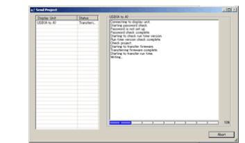
10. When transfer is completed, the state of the dialog box changes from [Transferring] to [Transfer Complete]. Click [Close].
