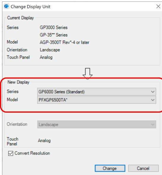
Change the Display unit from GP3000 Series to GP6000 Series (Standard).
