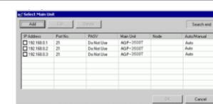
6. Select each IP address of the display unit to which you want to transfer and click [OK]. When multiple IP addresses are checked, the project is sent to multiple display units at once.
