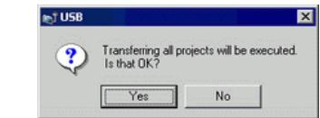
9. The transfer begins. The following dialog box appears during transfer, and you can check the communication status. (The display unit changes to Transferring mode and communication with the device/PLC is suspended.)
