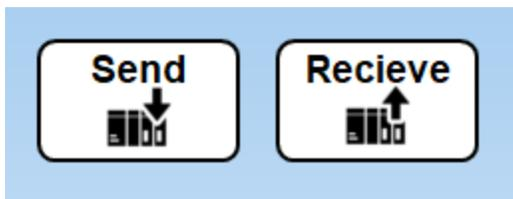
Send uses the DBSelect Command to read up the values of the selected recipe from the database and transfers it to the sudo-PLC variables.
