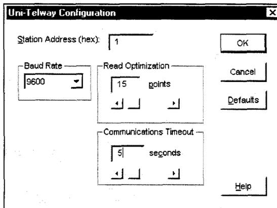
Figure 3. Uni-Telway Configuration dialog box
