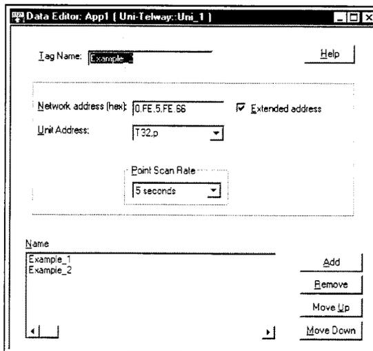
Figure 6. Uni-Telway Addressing, Example 2
