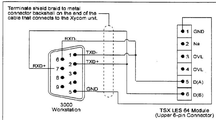
Figure 1. RS-485 Pinout
