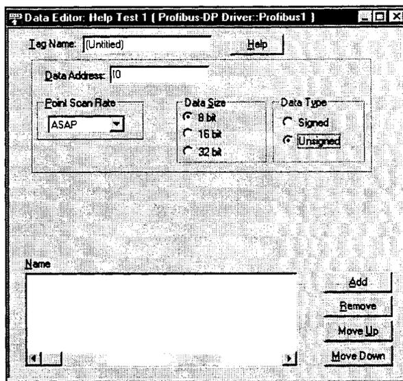
Figure 5. Profibus-DP Data Point Configuration Form
