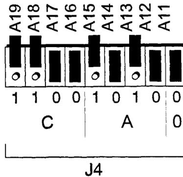
Figure 2. Memory Address Configuration Example
