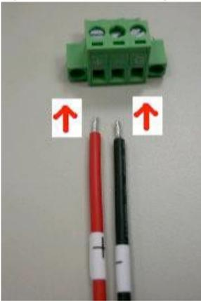
2) Screw the Terminal block to fix the cable.
