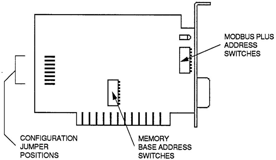
Figure B-3. SA85 Network Adapter Board Layout
