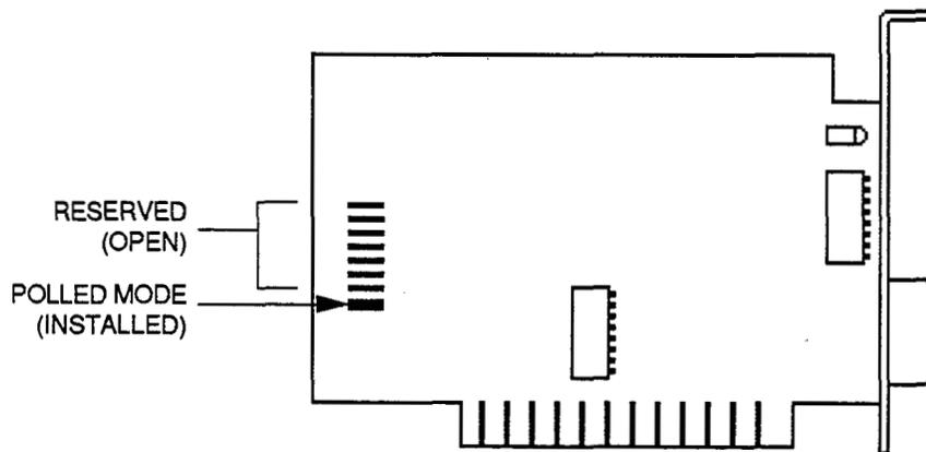
Figure B-7. SA85 Configuration Jumper Setting
