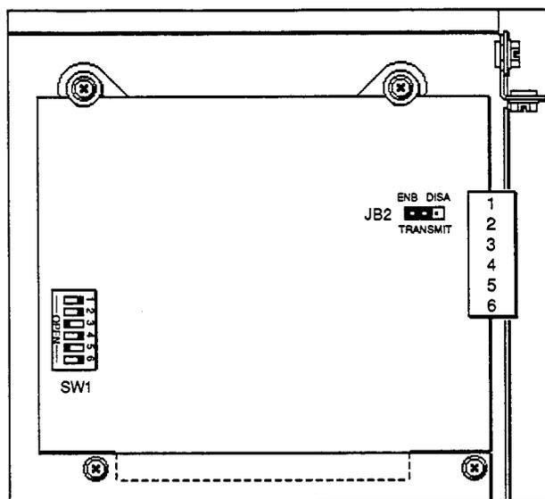
Figure C-1. Direct Connect Adapter Card Jumper and Switch
