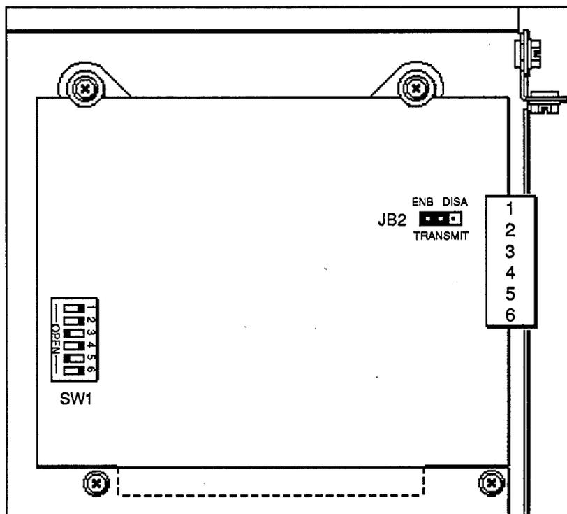
Figure A-1. Direct Connect Adapter Card Jumper and Switch
