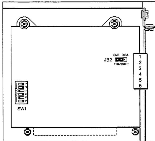
Figure D-1. Direct Connect Adapter Card Jumper and Switch
