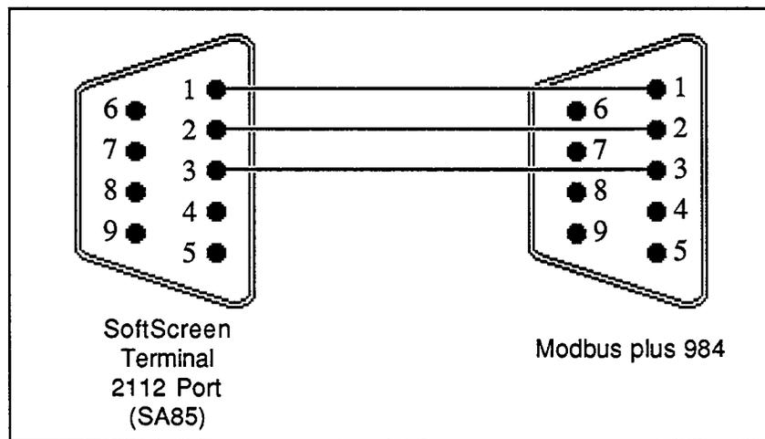
Figure B-1. Cabling to the Modbus Plus 984
