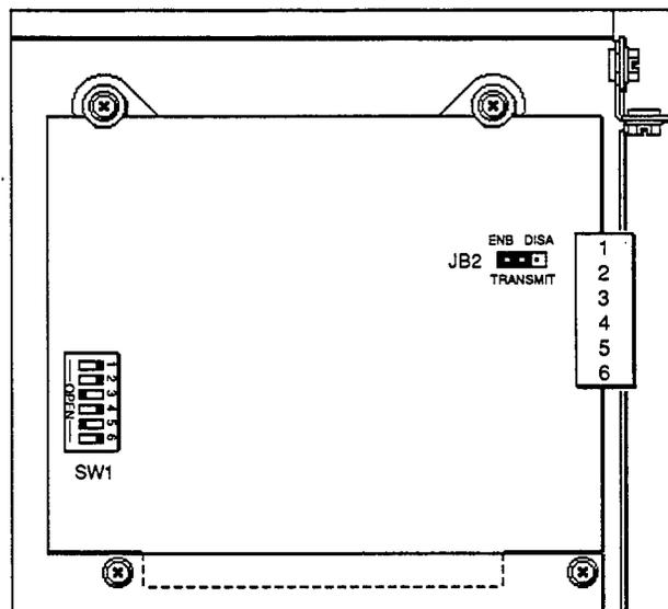
Figure E-1. Direct Connect Adapter Card Jumper and Switch
