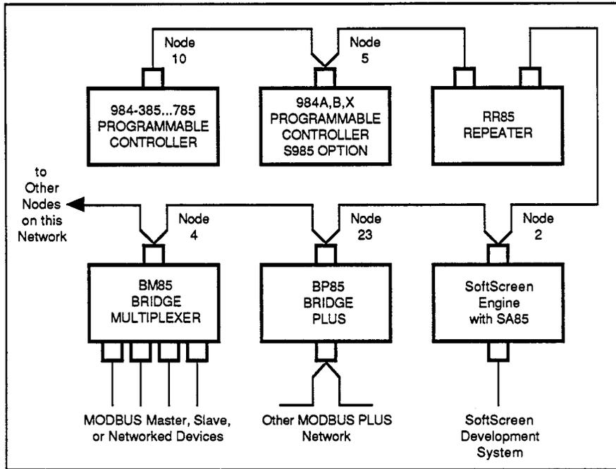
Figure B-2. Modbus Plus Network Configuration Example
