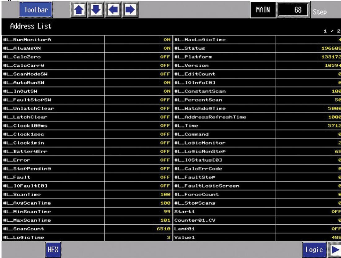
The Right Arrow button (lower right hand corner of both Logic and Address List screens) takes you to the toolbar as shown in Fig. 3c. Use this toolbar to exit the Ladder Monitor or use the “STOP” button to stop and restart logic execution.
