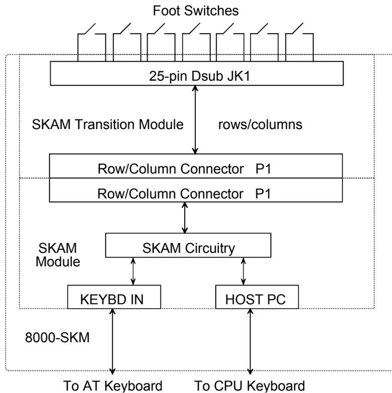
Figure Chapter 1 -1. 8000-SKM Block Diagram
