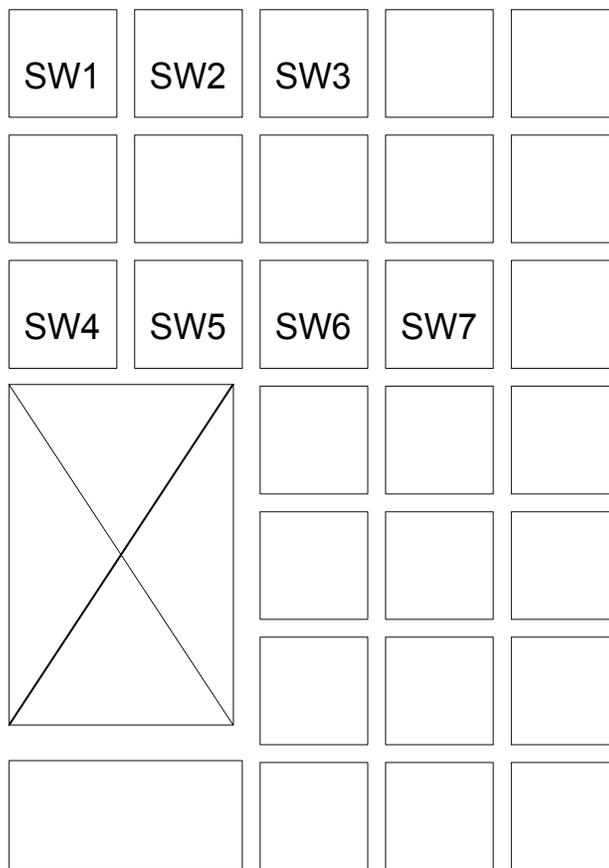
Figure Chapter 3 -1. Switch Locations on 9450 Keypad
