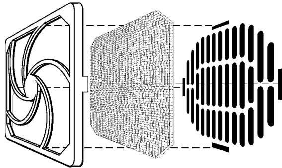
Figure 5-1. Fan Assembly
