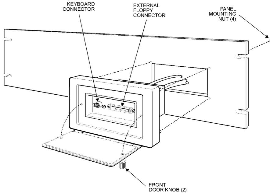
Figure 3-12. Front Floppy and Keyboard Access Option
