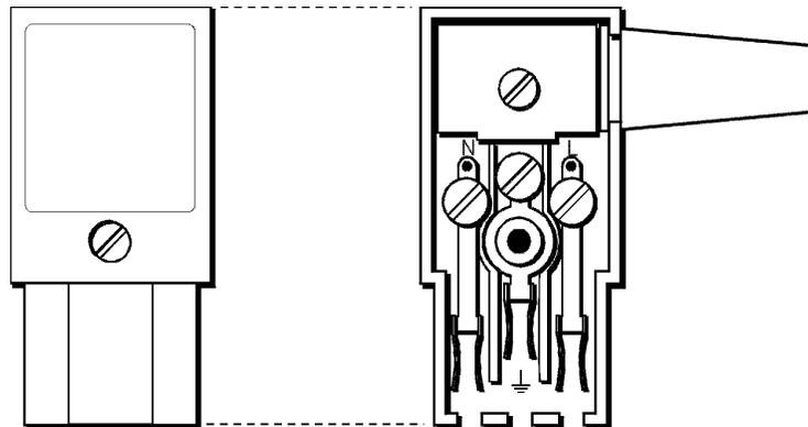
Figure 3-20. Internal View of 3515 AC Power Connector
