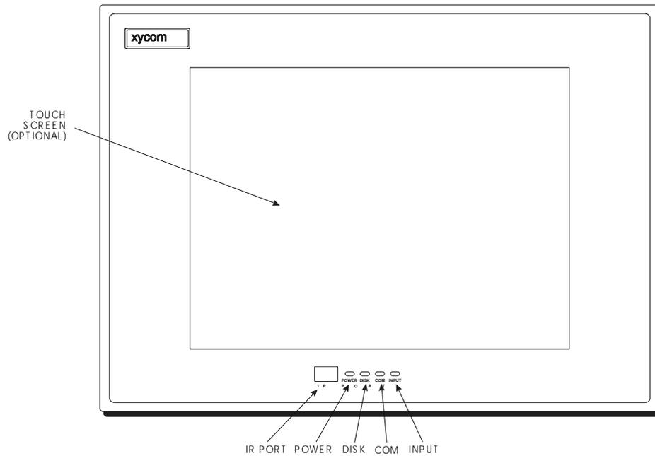
Figure 3-1. 3515 TFT Active Display Front Panel
