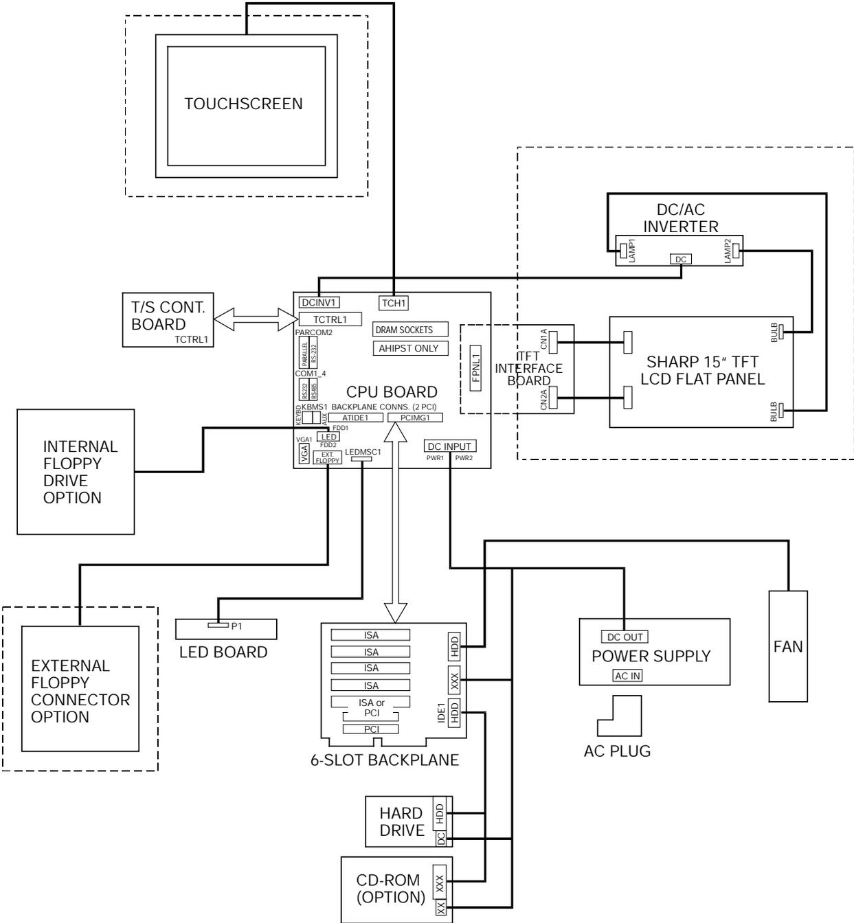
Figure B- 1. 3515 TFT System Block Diagram
