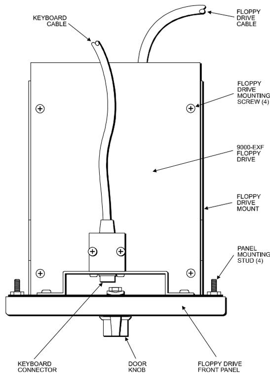
Figure 3-10. Floppy Drive - Front Mounting Option (top view)
