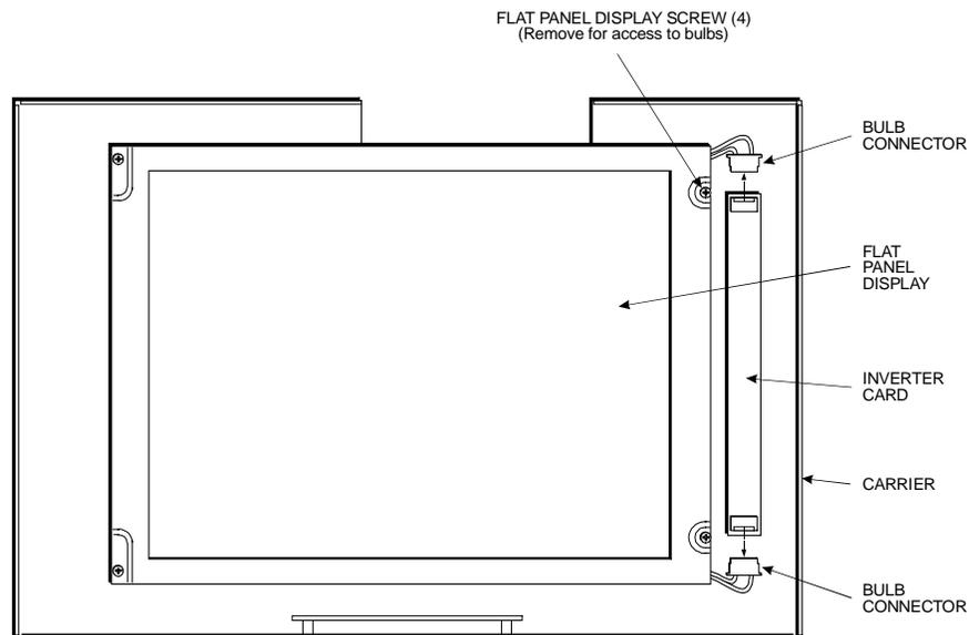
Figure D- 1. Model #LQ150X1DG16 - Front View
