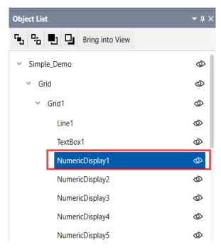
2. In Properties tab, select **Function > Basic > Current Value** and bind the desired variable from variable selector.
