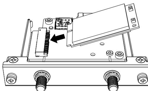
3. Push the 4G mini PCIe card from above and secure it with the screws removed in step 1.
