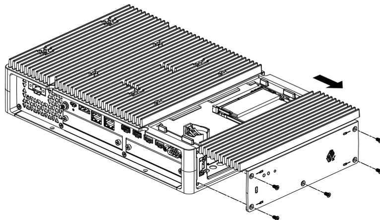
4. When equipped with M.2 SSD, remove the heat sink and heat sink pad (for top) before installing the FAN kit. For information on the heat sink and heat sink pad for M.2 SSD, see M.2 SSD Installation, page 97.
