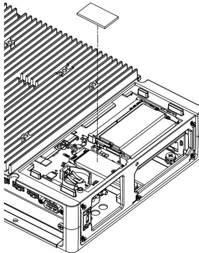
9. Put in the heat sink, and attach with screws.
