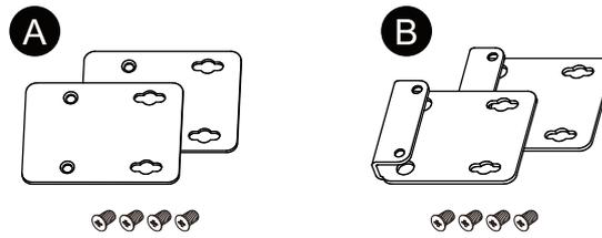
2. Remove the screws attached to the product (4 pieces), then use the screws for the book mount adapter to attach it to the product. When attaching to the top of the product, attach the B book mount adapter so that the protruding part faces the product.
