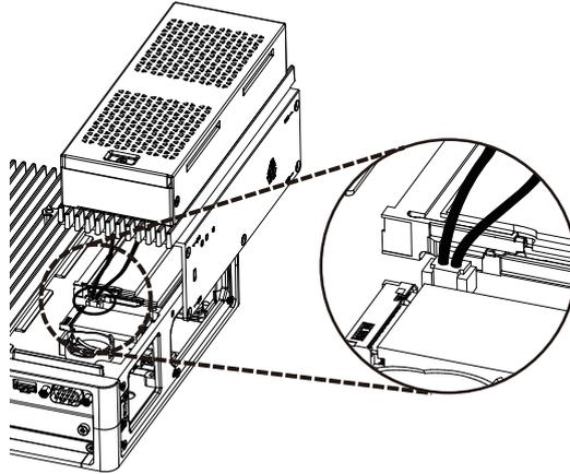
6. Using the screws removed in step 3, secure the FAN kit.
