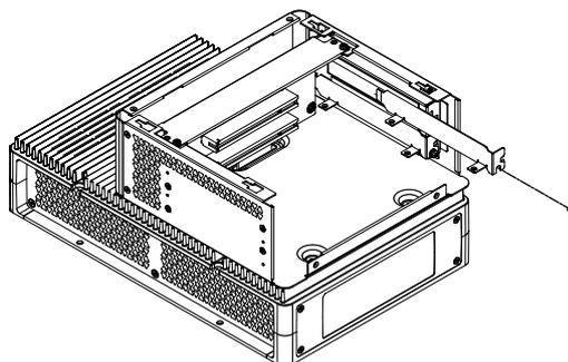
6. Insert the PCI/PCIe card, and secure the card with the screw removed in step 5.
