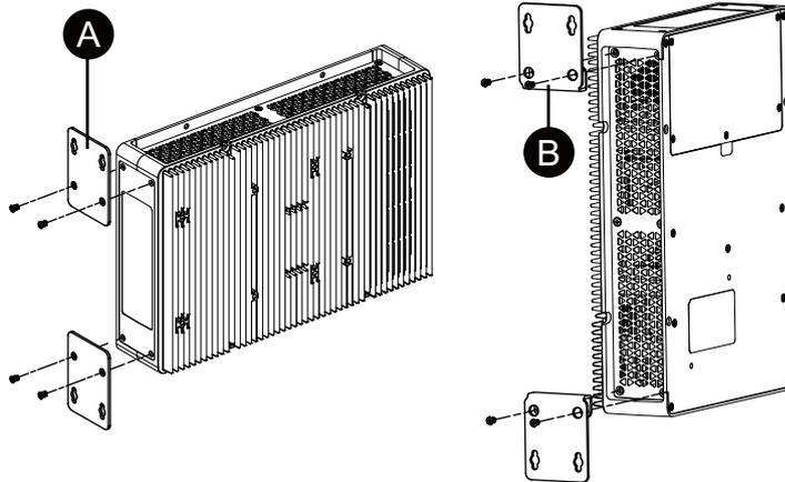
3. Install the product to the panel or wall with M4 screws (4 pieces).
