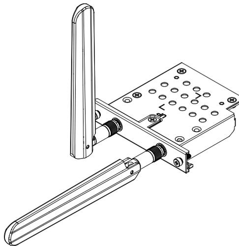
You can attach the antenna to the outside of the panel using the following optional cable.
