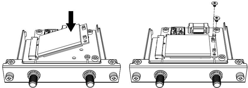
4. As shown below, plug the antenna cable connector securely to the connector on the 4G mini PCIe card. Looking from above the interface, plug the cable connector on the left side to connector 1, and the cable connector on the right side to connector 2.
