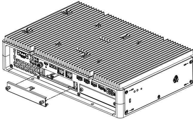
4. With the side labelled “UP” facing upward, insert the optional interface into the Box Module and tighten the screws.
