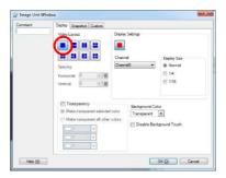
8) In the [Display] area, click one screen mark, and under the [Channel], select the camera image to be displayed in this upper left area (for example, Channel 0).
