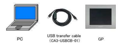
(1) Connect your PC and the GP unit of GP4000 series with a USB transfer cable. If the driver of the cable has not been installed on you PC, a dialog box will appear. Please follow the instructions.
