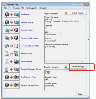
(2) Make sure that the [Device] in the "Transfer Settings Information" is set to [USB]. If not, click the [Transfer Setting] button to open the "Transfer Setting" dialog box. Select [USB] in the Communication Port Settings field and click [OK].
