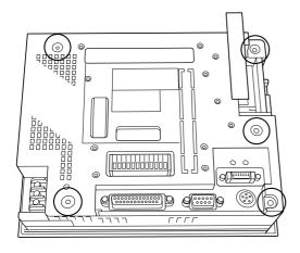
1) Turn OFF the GP/PS unit's power supply. Open the CF Card's cover and unscrew the unit's five (5) Rear Cover attachment screws.
