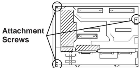
3) Loosen the three (3) circuit board attachment screws.
