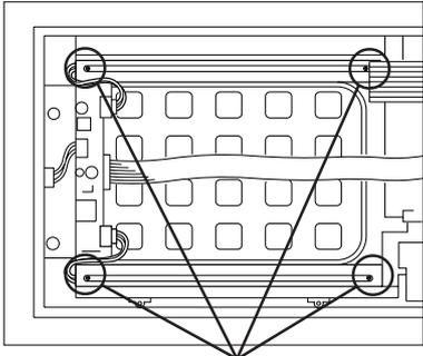
4) Loosen the upper and lower backlight holder attachment screws, and remove the upper backlight unit's metal cover.
