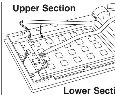
If the backlight has an arrow here, it is used only for the upper backlight.
