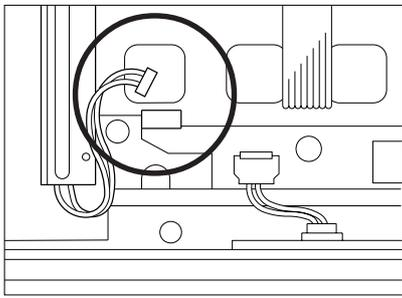
3) Disconnect the upper backlight's power connector.
