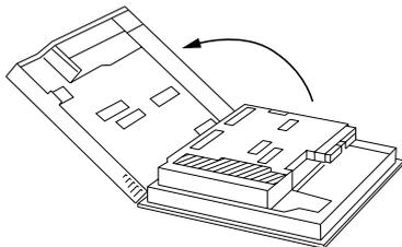
1) Turn the GP's power OFF (i.e. disconnect the GP's power cord). Remove the three (3) I/F covers, and use a Phillips screwdriver to remove the case's seven (7) rear attachment screws. Pivot the rear cover open, starting from the top of the unit.
