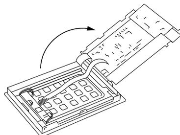
4) The circuit board is attached on one side, and hinges open.
