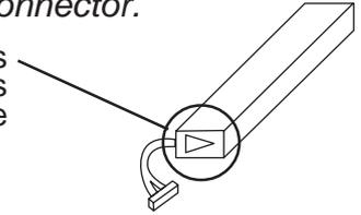
7) Insert the metal cover's three (3) positioning tabs into the backlight holder's positioning slots. Next, insert and tighten the cover's two (2) attachment screws.
