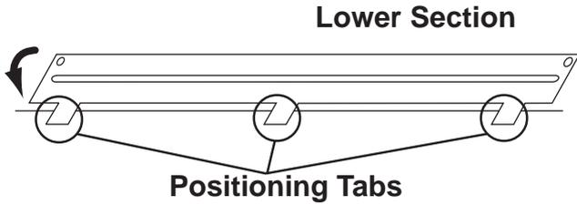
6) Insert the new backlight into the GP/GLC.
