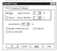
When you set parameters on the [**Tuning**] tab, you are setting the parameters the ladder logic program uses when it is written to the GLC Controller. Subsequently, whenever this particular program is run, the GLC Controller will use these settings, unless they are changed manually. These settings are unique to this program.
