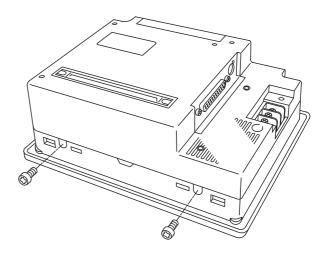
3) Pull the unit's Rear Cover straight up to remove it.
