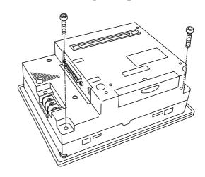
2) Remove the unit's two (2) top face attachment screws.
