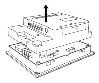
4) Detach the backlight unit's power connector from the display module by grasping both of the connector's removal prongs and pulling gently upwards.
