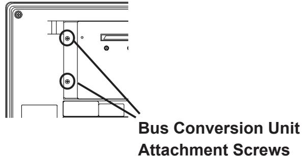
6. Attach an expansion unit to the Bus Conversion unit and tighten the three (3) expansion unit attachment screws (included with this unit).
