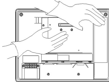
5. Reattach the conversion unit's attachment screws and secure it to the GLC.
