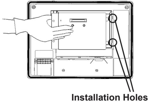
4. Hold the GLC with your left hand and press the Bus Conversion unit into its slot with your right hand. Be sure that the unit is seated correctly in place, so that no gaps remain between the GLC and the Bus Conversion unit.
