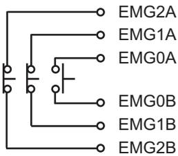
**NOTE:** When using a model without an emergency stop switch or a stop switch, disconnect (NC) these signal lines.
