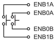
**NOTE:** The contact is OFF when the switch is pressed to the innermost position then returned to the not pressed position.
