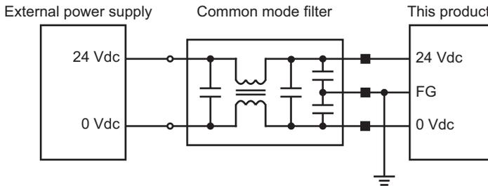
■ The black square indicates the connection point for the direct-connect cable and common field filter.
