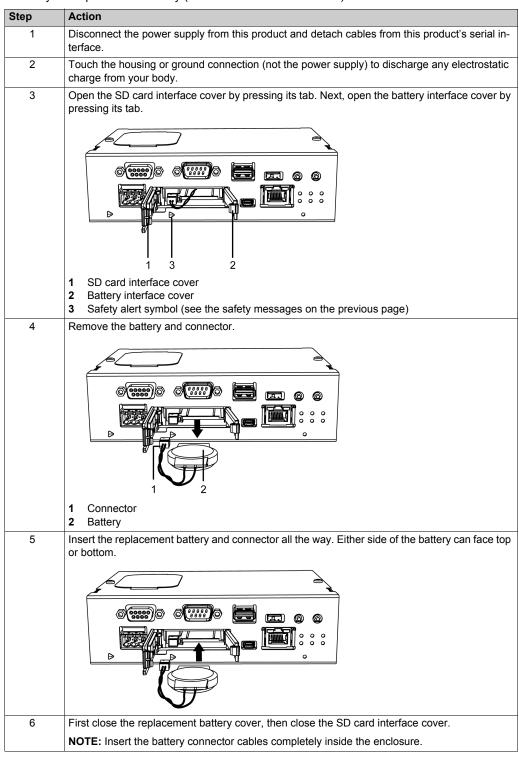
**NOTE?** After reconnecting the power supply, set up the clock again. Refer to your screen editing software manual on how to set up the clock.
