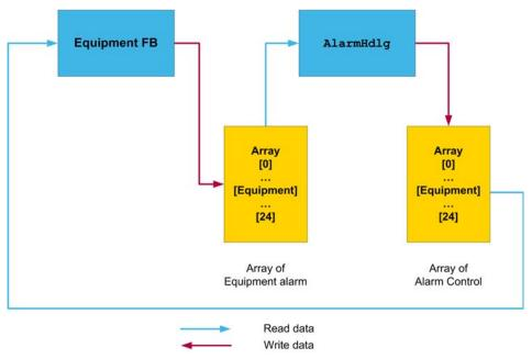
The AlrmHdlg FB uses arrays of structures to exchange the data between TurnTable and AlrmHdlg function block. Each array element is representing one equipment in the conveying line. The index of this array (symbolized in the table below with  $\mathbf{x}$ ) is unique and must be kept through out the entire application.
