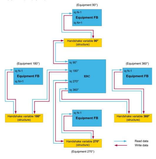
On one hand, the ERC FB needs to read from the structure the relevant information from the neighboring equipment, on the other hand the ERC FB has to write its own status in the same structure (handshake variable). In order to share this information by using the identical structure, one variable for each direction needs to be defined.
