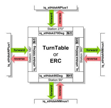
In some conveying applications it is needed to link handshake pins of the same type (N+1 or N-1) together for stations which are neighboured to a turntable or a transfer table (ERC = Eccentric Roller Conveyor). In this case the logical direction of the handshake pins on a TurnTable or an ERC function block can be switched between the types N+1 and N-1. Therefore the configuration parameters of the sub-structure stConfOfHdskSwap are provided.
