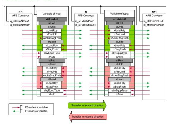
The handshake mechanism works considering a predefined transfer direction. That means, a pin of type iq\_stHdskNMnus1 must be linked with a pin of type iq\_stHdskNPlus1.
