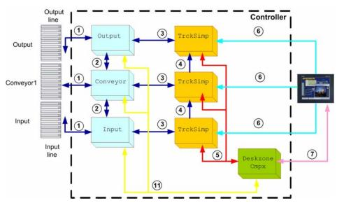
Use Case 2 - With Tracking Function and Without Alarm Management Function
