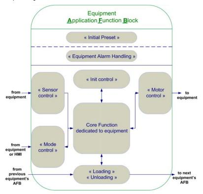
The equipment application function blocks are built with some common functions as described below:
