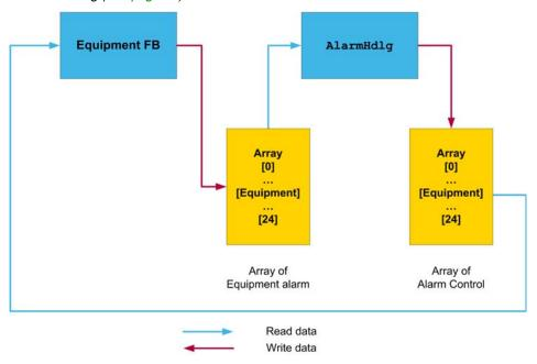
The AlrmHdlg FB uses arrays of structures to exchange the data between Output and AlrmHdlg function block. Each array element is representing one equipment in the conveying line. The index of this array (symbolized in the table below with  $\mathbf{x}$ ) is unique and must be kept through out the entire application.
