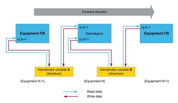
On one hand, the <code>Conveyor</code> FB needs to read from the structure the relevant information from the neighboring equipment, on the other hand the <code>Conveyor</code> FB has to write its own status in the same structure (handshake variable). In order to share this information by using the identical structure, one variable for each direction needs to be defined.
