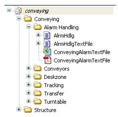
To be language independent, the function blocks of the Conveying Library support unique alarm and alert IDs with a value ranging from 0...255. Using the alarm textfiles the ID can be combined with the corresponding message in the HMI application.
