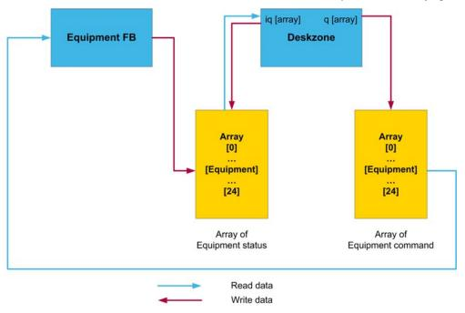
The Deskzone FB uses arrays of structures to exchange the data between TurnTable and Deskzone function block. Each array element is representing one equipment in the conveying line. The index of this array (symbolized in the table below with  $\mathbf{x}$ ) is unique and must be kept through out the entire application
