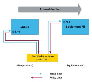
On one hand, the Input FB needs to read from the structure the relevant information from the neighboring equipment, on the other hand the Input FB has to write its own status in the same structure (handshake variable). In order to share this information by using the identical structure, one variable for each direction needs to be defined.
