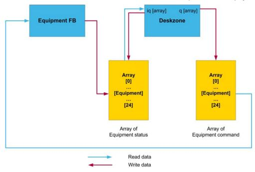
The Deskzone FB uses arrays of structures to exchange the data between ERC and Deskzone function block. Each array element is representing one equipment in the conveying line. The index of this array (symbolized in the table below with  $\mathbf{x}$ ) is unique and must be kept through out the entire application
