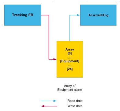
The AlrmHdlg FB uses arrays of structures to exchange the data between TrckCmpx and AlrmHdlg function block. Each array element is representing one equipment in the conveying line. The index of this array (symbolized in the table below with  $\mathbf{x}$ ) is unique and must be kept through out the entire application.
