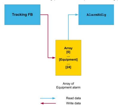
The AlrmHdlg FB uses arrays of structures to exchange the data between TrckSimp and AlrmHdlg function block. Each array element is representing one equipment in the conveying line. The index of this array (symbolized in the table below with  $\mathbf{x}$ ) is unique and must be kept through out the entire application.
