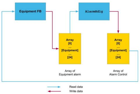
The AlrmHdlg FB uses arrays of structures to exchange the data between Input and AlrmHdlg function block. Each array element is representing one equipment in the conveying line. The index of this array (symbolized in the table below with **x**) is unique and must be kept through out the entire application.
