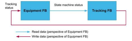
As the designated pins can be directly linked (from Equipment to TrckSimp and vice versa), no variable between these 2 FBs is necessary.
