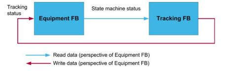
As the designated pins can be directly linked (from Equipment to TrckCmpx and vice versa), no variable between these 2 FBs is necessary.
