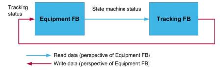
As the designated pins can be directly linked (from ERC to TrckCmpx and vice versa), no variable between these 2 FBs is necessary.
