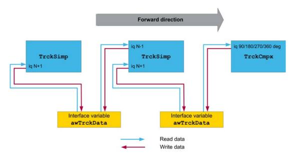
On one hand, the TrckSimp FB needs to read the data during the loading process, on the other hand the TrckSimp FB has to write the data during the unloading process. In order to transfer the data by using the identical interface variable, one variable for each direction needs to be defined.
