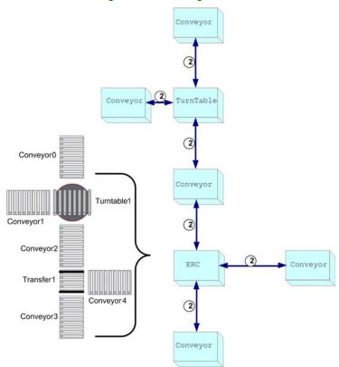
2 Link to manage handshaking function between AFBs to follow goods on the conveying line
