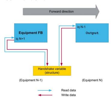
On one hand, the <code>Output</code> FB needs to read from the structure the relevant information from the neighboring equipment, on the other hand the <code>Output</code> FB has to write its own status in the same structure (handshake variable). In order to share this information by using the identical structure, one variable for each direction needs to be defined.
