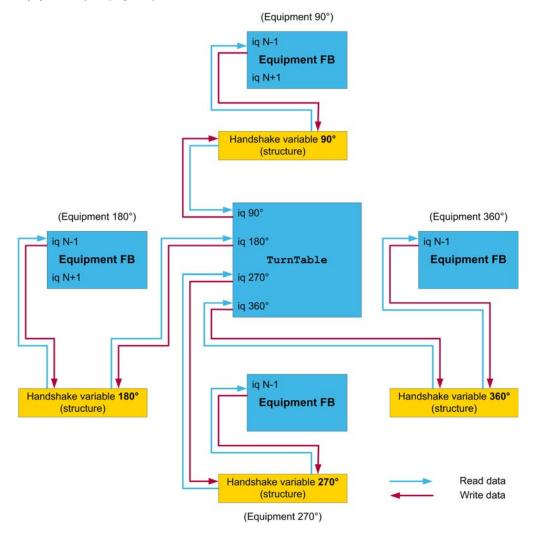
On one hand, the TurnTable FB needs to read from the structure the relevant information from the neighboring equipment, on the other hand the TurnTable FB has to write its own status in the same structure (handshake variable). In order to share this information by using the identical structure, one variable for each direction needs to be defined.
