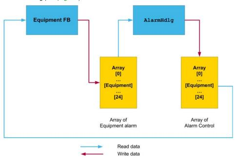
The AlrmHdlg FB uses arrays of structures to exchange the data between ERC and AlrmHdlg function block. Each array element is representing one equipment in the conveying line. The index of this array (symbolized in the table below with **x**) is unique and must be kept through out the entire application.
