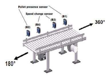
If the Conveyor is used to deliver in 360° direction (considered in general as forward), only sensors B1 and B3 are taking effect on the function of the Conveyor. As B3 sensor is merely used to change the speed of the pallet, this sensor is only applicable for Conveyors which support two speeds. All sensors are wired to OTBs which are providing their status by the OTB structures with the input <code>i\_stOtbIput</code>.
