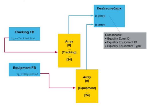
The DeskzoneCmpx FB uses arrays of structures to link the data with the Equipment and Tracking function blocks. Each array element is representing one equipment in the conveying line. The index of this array (symbolized in the table below with  $\mathbf{x}$ ) is unique and must be kept through out the entire application
