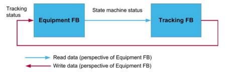
As the designated pins can be directly linked (from Output to TrckSimp and vice versa), no variable between these 2 FBs is necessary.
