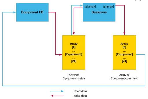
The Deskzone FB uses arrays of structures to exchange the data between Output and Deskzone function block. Each array element is representing one equipment in the conveying line. The index of this array (symbolized in the table below with  $\mathbf{x}$ ) is unique and must be kept through out the entire application
