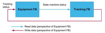
As the designated pins can be directly linked (from Input to TrckSimp and vice versa), no variable between these 2 FBs is necessary.
