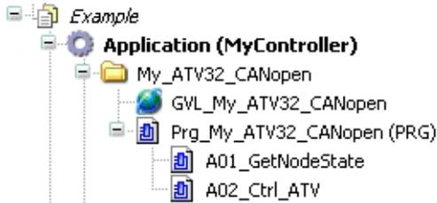
The Program (PRG) as part of a Device Module is added automatically to the task configuration of the project.
