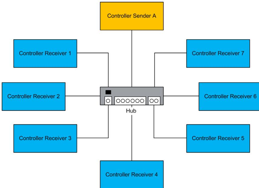
**Controller Sender A:** Sender with the global variables list (GVL) and receiver controller with global network variables lists (GNVLs)
