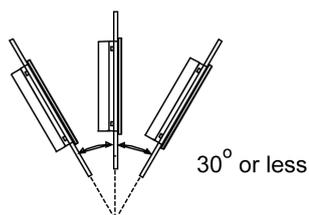
When installing this product in a slanted position with an incline more than 30°, the ambient temperature must not exceed 40 °C (104 °F). You may need to use forced air cooling (fan, A/C) to ensure the ambient operating temperature is 40 °C or less (104 °F or less).
