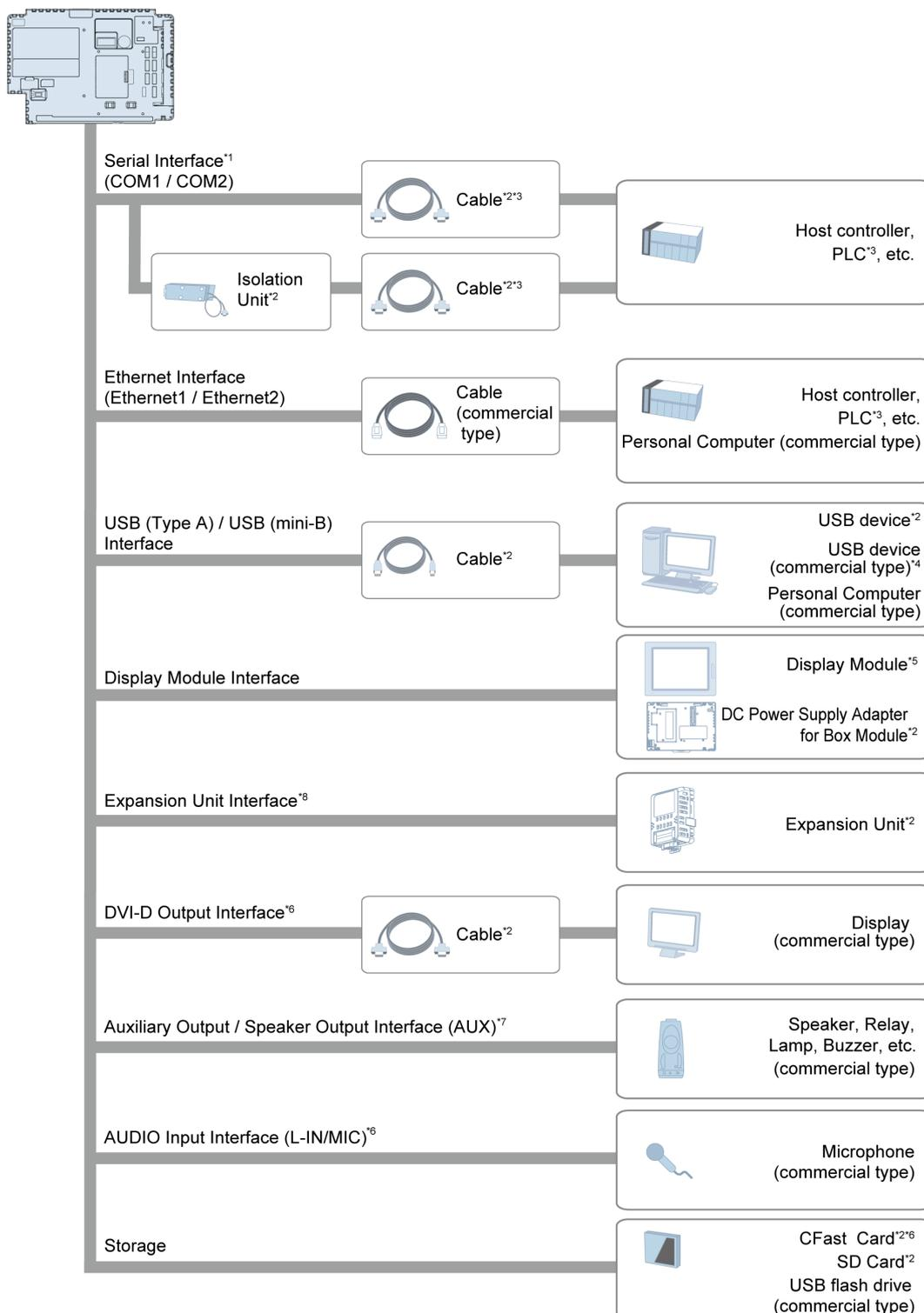
\*1 In order to use this as an isolation port, Isolation Unit is required. To use RS-232C isolation unit, set the #9 pin of the COM port to VCC (on Standard Box, connect the isolation unit to COM1).
