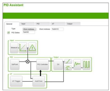
By using the PID Assistant, the PID 0 is configured and memory words are mapped to different functions. This table describes the memory addresses used in the PID Assistant:
