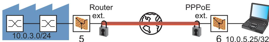
Figure 44: Connecting a PC with a subnetwork via a public network
