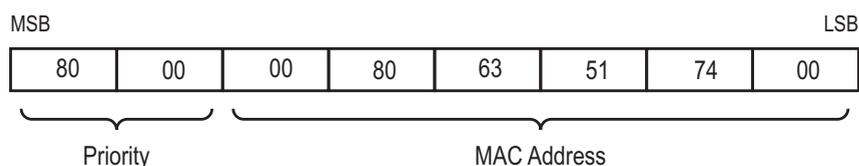
Figure 40: Bridge Identifier, Example (values in hexadecimal notation)
