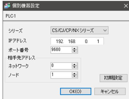
個別機器設定 dialog box showing settings for PLC1. The series is set to CS/CJ/CP/NX series. The IP address is 192.168.0.1, port is 9600, network is 0, and node is 1. There are buttons for '初期設定', 'OK(O)', and 'キャンセル'.
