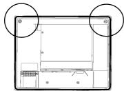
Turn the GP's power OFF (i.e. disconnect the GP's power cord). Use a Phillips screwdriver to remove the case's two rear attachment screws, and pivot the rear cover open, starting from the top of the unit.
