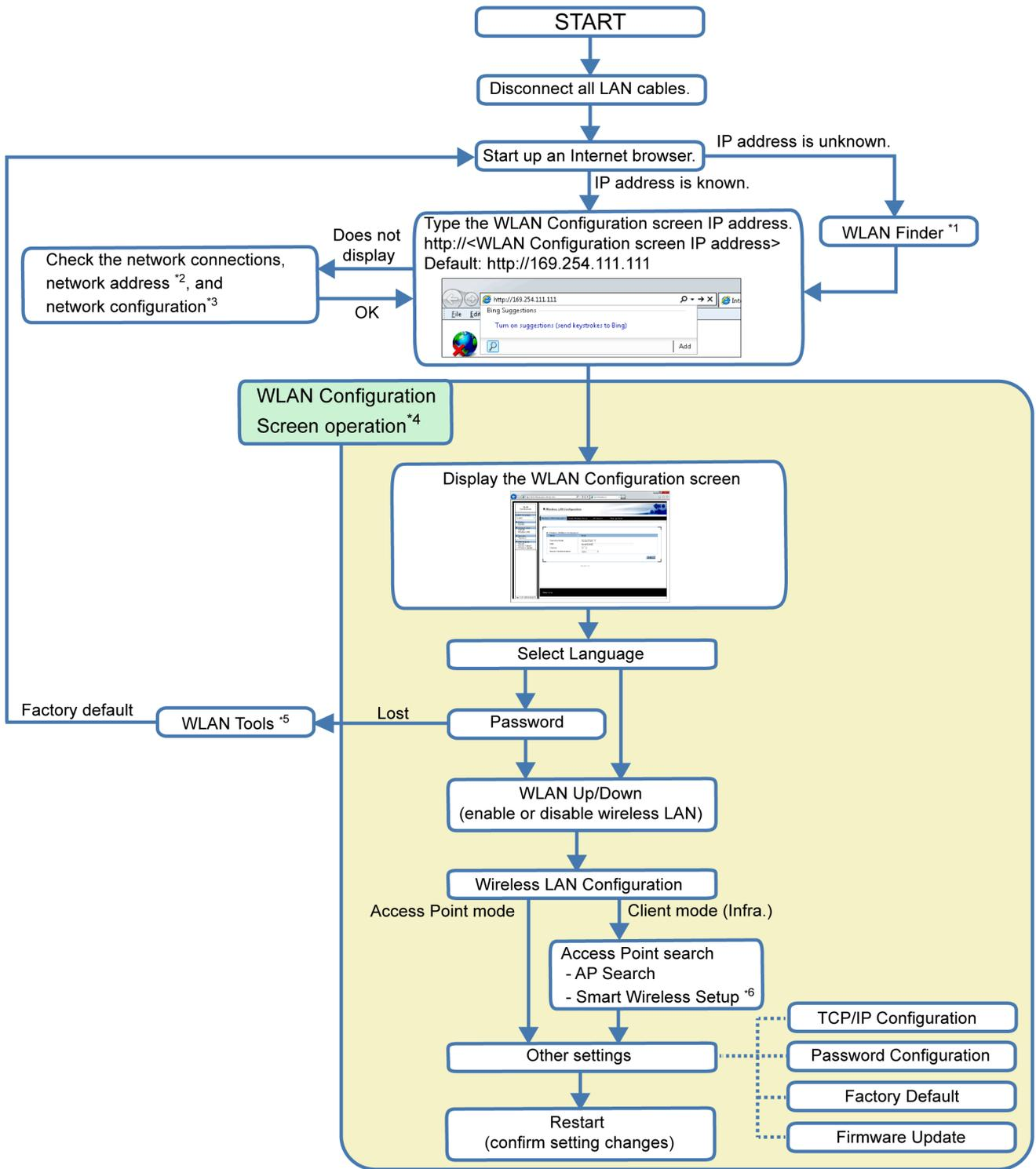
\*1 If the IP address is unknown, you can use the WLAN Finder to search for the IP address. You can conduct a search when the Open Box wireless LAN network adapter and the wireless LAN model are on the same network. You can download the WLAN Finder from our website at <http://www.pro-face.com/trans/en/manual/1001.html>.
