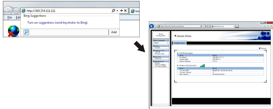
**NOTE:** If the WLAN Configuration screen IP address has already been edited using **TCP/IP Configuration**, page 17, enter the edited IP address. To display the WLAN Configuration screen with the new IP address, the WLAN Configuration screen and Local Area Connection network addresses must be the same.
