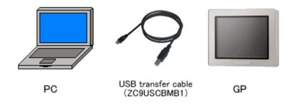
(1) Connect your PC and the GP unit with a USB transfer cable (model: ZC9USCBMB1). If the driver of the cable has not been installed on you PC, a dialog box will appear. Please follow the instructions.
