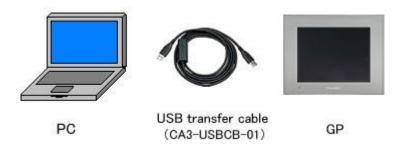
(2) Make sure that the [Device] in the "Transfer Settings Information" is set to [USB]. If not, click the [Transfer Setting] button to open the "Transfer Setting" dialog box. Select [USB] in the Communication Port Settings field and click [OK].
