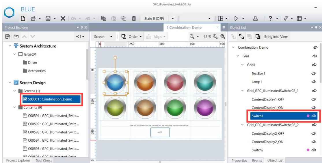
2. In Properties tab, select Function > Touch > Operation > Destination and bind the desired variable from variable selector.
