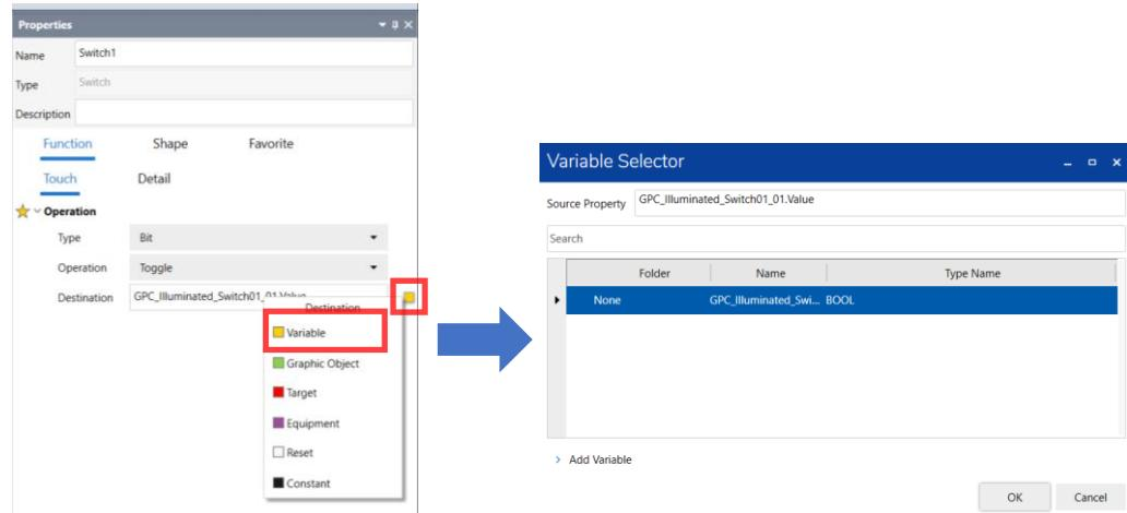
3. In Screen, select ContentDisplay(x)\_OFF. In Properties tab, select Shape > Size/Location > Visibility and bind the desired variable from variable selector.
